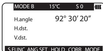
Press [F2] [ANG SET] to display the angle setting screen, then press [F4] [↑] to move the cursor to "2. H. ANGLE INPUT":
